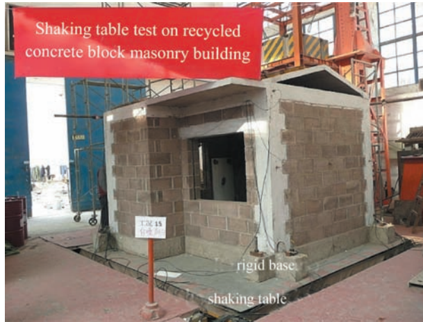
Fig. 13 General view of the RAC block masonry structure
