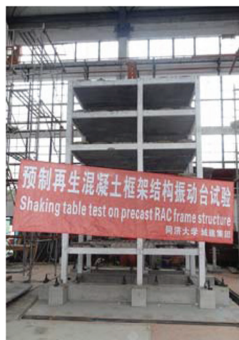
(b) Precast model on the shaking table
