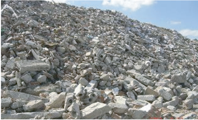
Figure 1. Demolition concrete produced RCA of model
