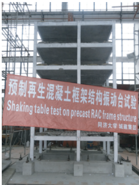
Figure 9. General view of precast RAC frame model
